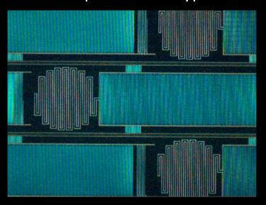
10 - 95 μm: Unit cell of mid-IR KID absorber.
